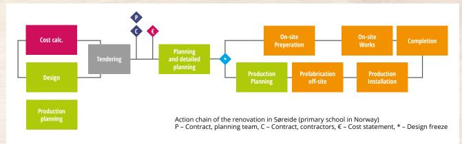
Figure 2: The best offer for the renovation of the primary school of Søreide in Norway based on the cooperation of the main contractor with the architects team. Contract conclusion (see "P" and "C") was followed by an extensive design phase "Planning and detailed planning", in which prefabricated elements and other solutions were optimized by architects, engineers and operating companies. (Source: Asplan Viak /NO)
